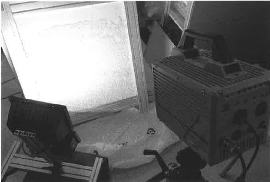
Figure 1. High-speed imaging measurement setup for crack propagation study in tempered glass.
