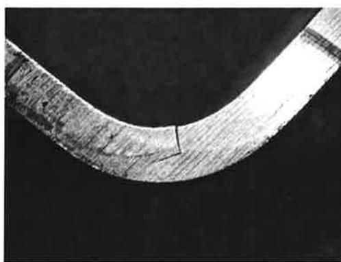
Figure 5. Crack branching observed in a large scale laboratory specimen.
