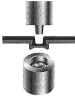
Fig. 1. A typical joint made by noncutting, single stroke clinching method.
