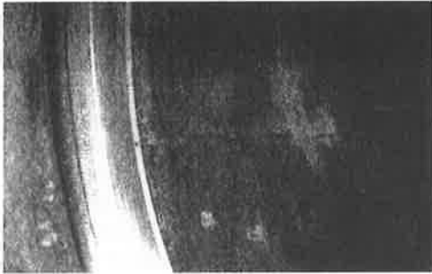
Figure 7. Cracked connecting rod. The total length of the crack is about 110 mm.
