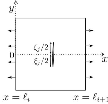
Figure 4. A central crack on a tensioned plate.
