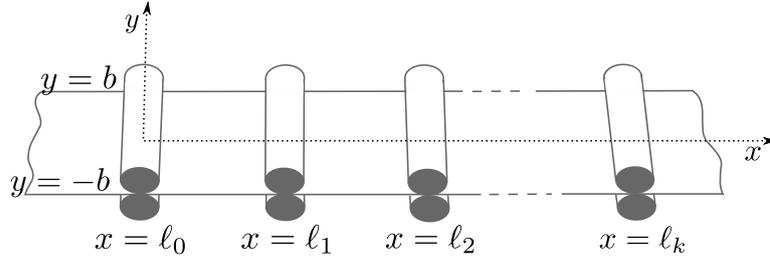
Figure 1. A band travelling in a system of rollers.
