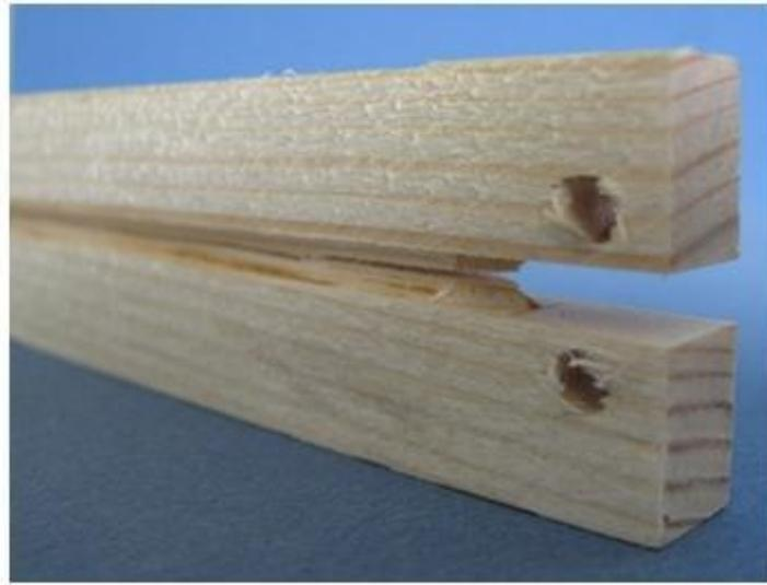
Figure 6. Modified DCB specimen: view of the RL crack propagation system.
