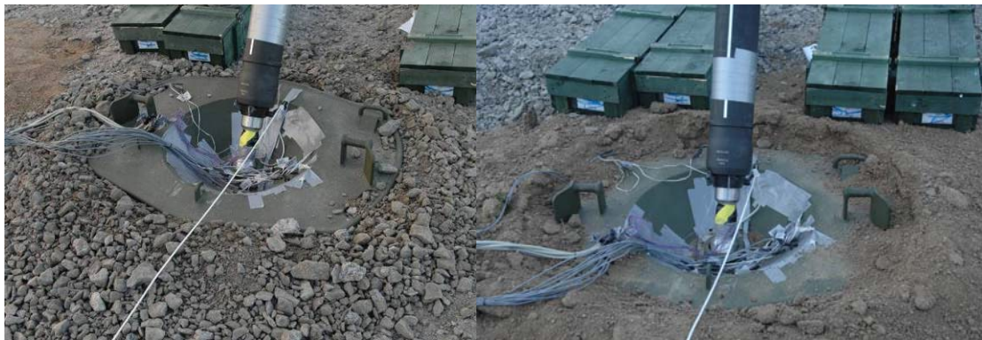
Figure 13. Base plate after service rounds firing on gravel soil (left) and on sandy soil (right).
