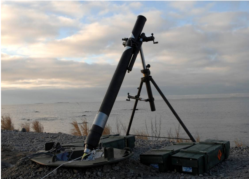
Figure 4. Traditional muzzle loaded 120 KRH 92 mortar on gravel soil before firing. The main components of mortar are: Base plate, special breech piece for socket force measurements, tube, sight unit and bipod assembly.
