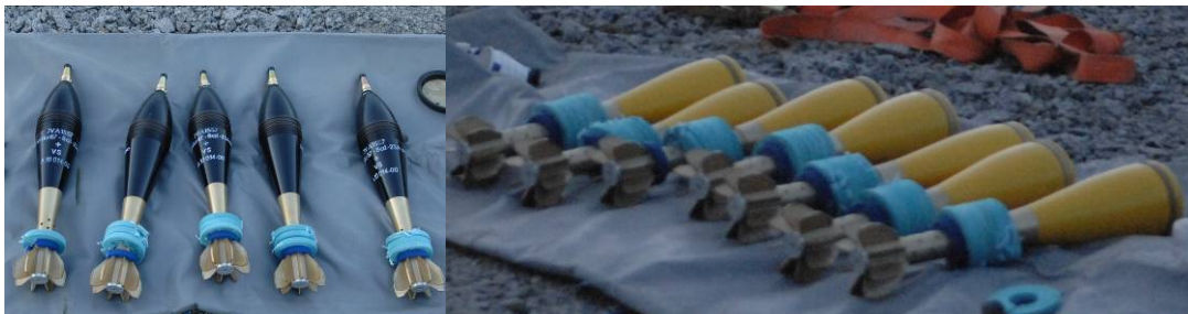
Figure 5. Traditional 120 mm HE shells (left) and ballistic slugs (right) with charge modules.
