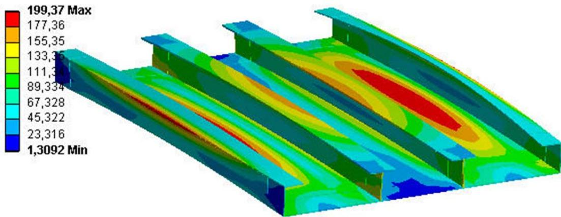
Figure 8. Von Mises stress distribution in the optimized structure. Maximum value 199.37 MPa contains only 0.3% estimation error compared to the target value of 200 MPa.
