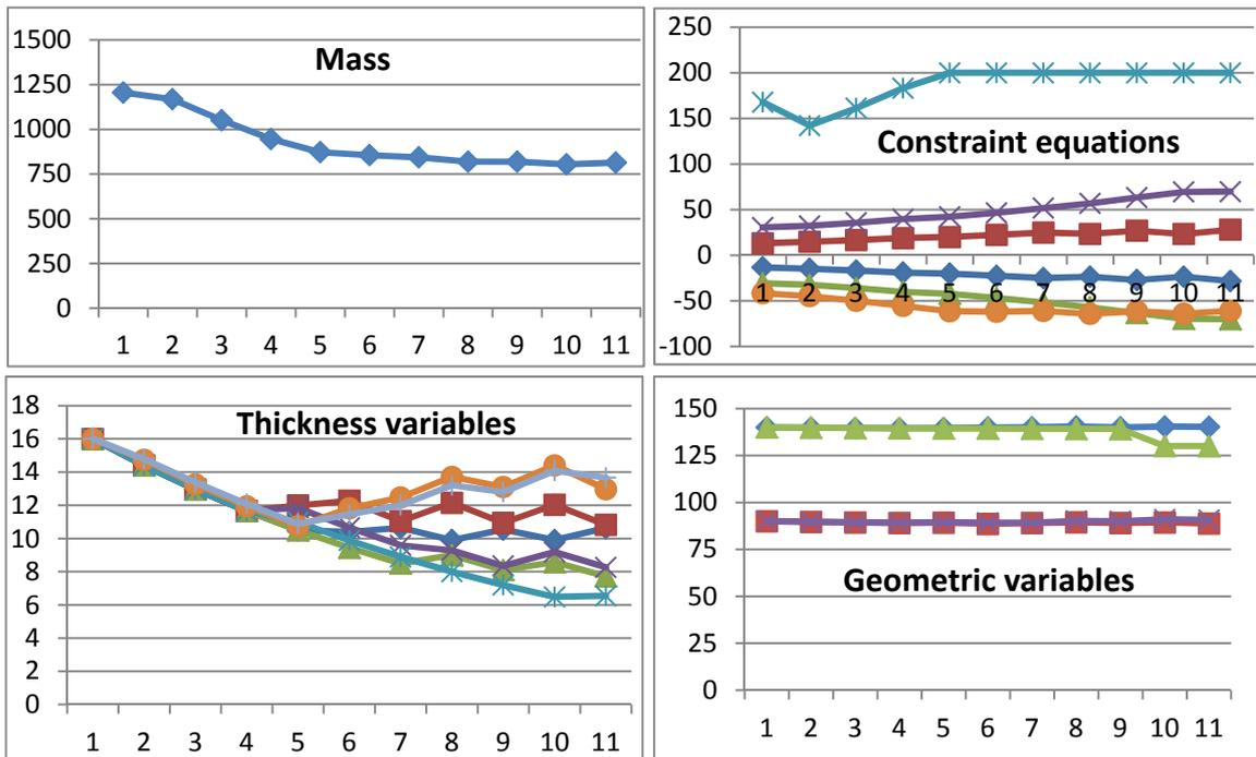
Figure 4. Convergence of the optimization iteration using RSM and linear surfaces.
