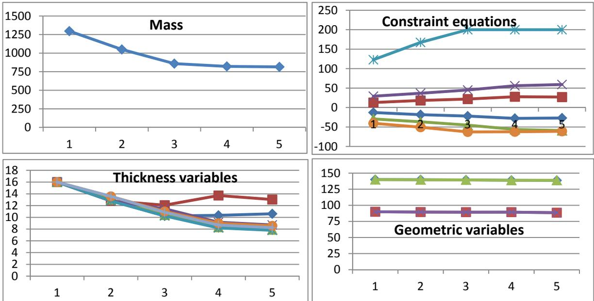
Figure 7. Convergence of the optimization iteration using Kriging method.
