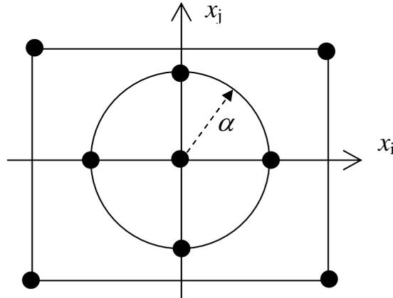
Figure 1. Central Composite Design test points in the case  $n = 2$ . Radius  $\alpha$ , that defines the axial points, can be chosen according to various optimality criteria [8,9].
