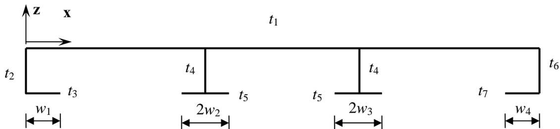
Figure 3. Design variables – seven thicknesses and four flange widths.
