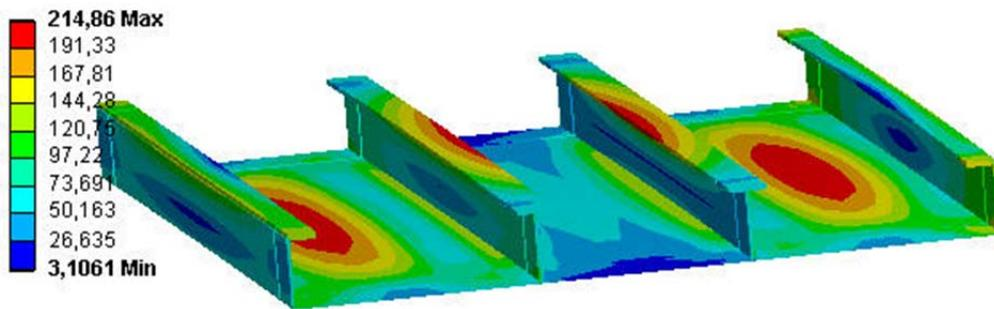
Figure 9. Von Mises stress distribution in the optimized structure. Maximum value 214.86 MPa contains 7,4% estimation error compared to the target value of 200 MPa.
