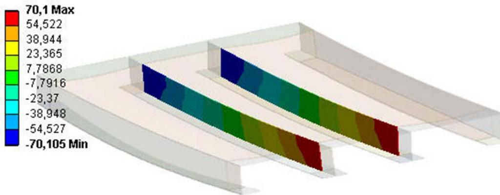
Figure 6. Shear stress distribution in the optimized structure at the central stiffeners. Maximum value 70.1 MPa contains only 0.1% estimation error compared to the target value of 70 MPa.
