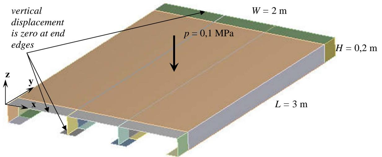
Figure 2. Loading, boundary conditions and dimensions of the stiffened plate.
