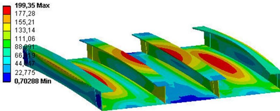
Figure 5. Von Mises stress distribution in the optimized structure. Maximum value 199.35 MPa contains only 0.3% estimation error compared to the target value of 200 MPa.
