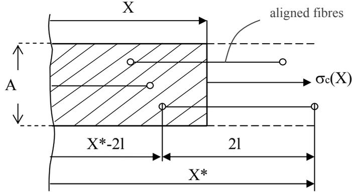
Figure 2. Fibre reinforced material, after Becker and Bürger (1975)
