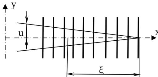
Figure 10. Crack growth in composite with short fibres
