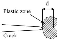
Figure 3. Plastic zone in front of the crack
