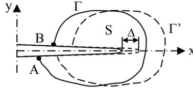
Figure 8. Propagation of a crack
