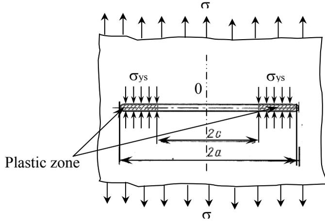
Figure 5. Stresses near the tips of a crack
