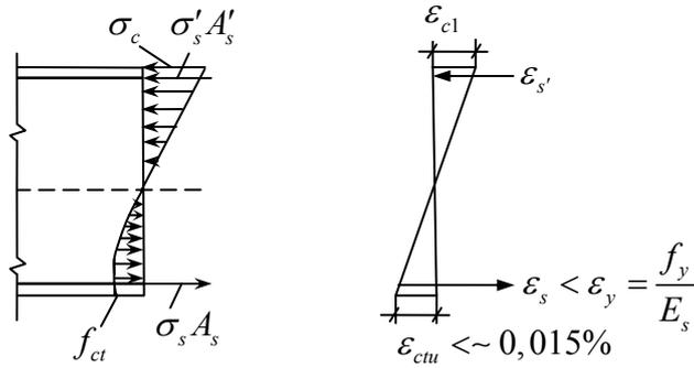
Figure 12. Stage one (I) of stress  $[\sigma]$  deformation  $[\varepsilon]$  state in reinforced concrete
