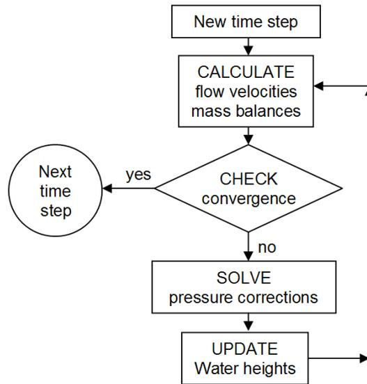
Figure 2. Flow chart for one time step
