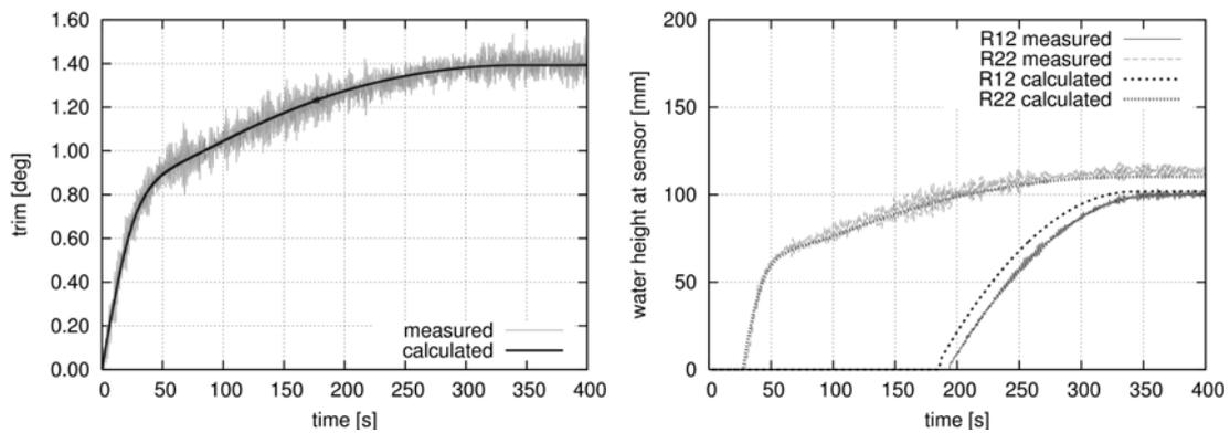
Figure 4. Examples of validation: trim angle and water levels in flooded compartments.
