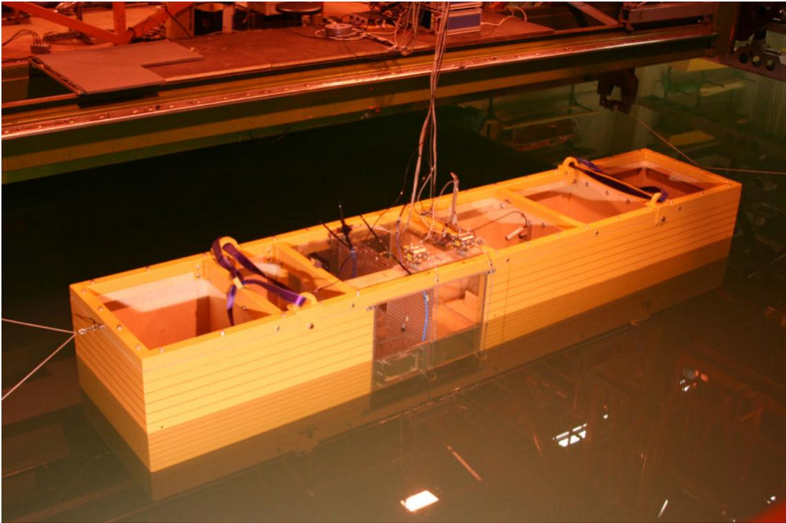
Figure 3. Model of the box-shaped barge
