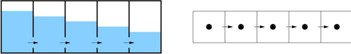
Figure 1. Staggered grid in flooding simulation
