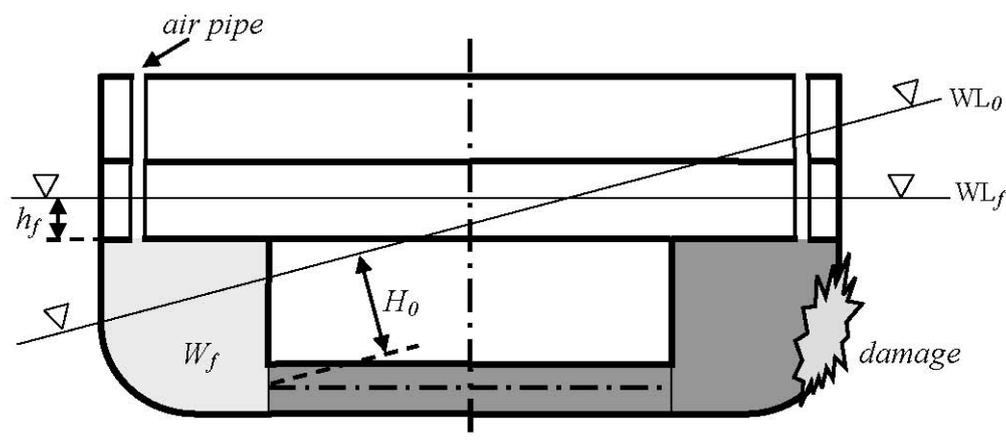
Figure 5. Definitions for cross-flooding; the initial condition is marked with subscript  $0$  and the final condition with  $f$
