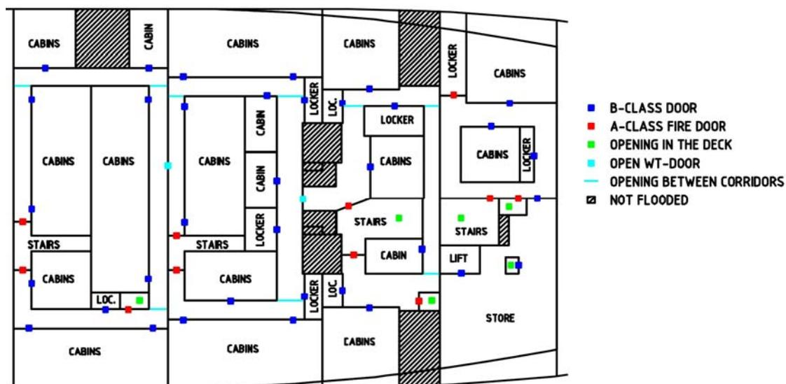
Figure 6. General arrangement of the flooded compartments
