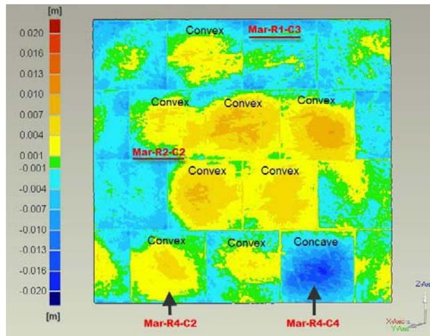
Figure 7. Terrestrial laser scanning data colouring by the magnitude of the deformation.
