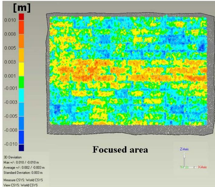
Figure 14. Delamination of bricks and the deterioration of joints detected from the laser scanning data.
