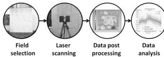
Figure 3. Flow chart of the laser scanning technique.
