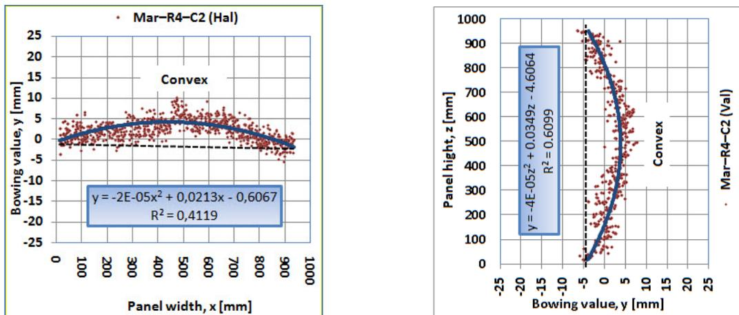
Figure 11. The horizontal and vertical bowing in marble panel Mar-R4-C2.
