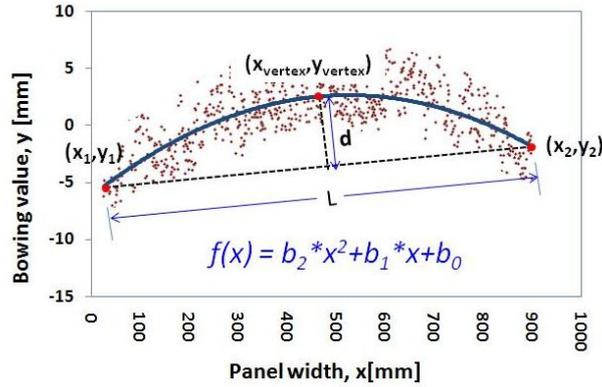
Figure 6. Example of the polynomial curve fitting of the point cloud data.
