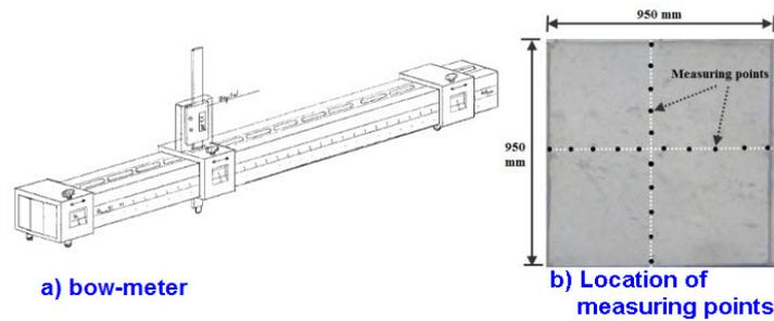
Figure 5. Manual measurement of the bowing of marble panels.
