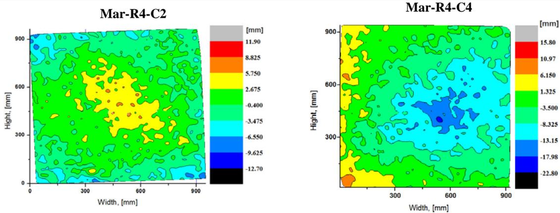
Figure 10. Terrestrial laser scanning data colouring by the magnitude of the bowing of the panel.
