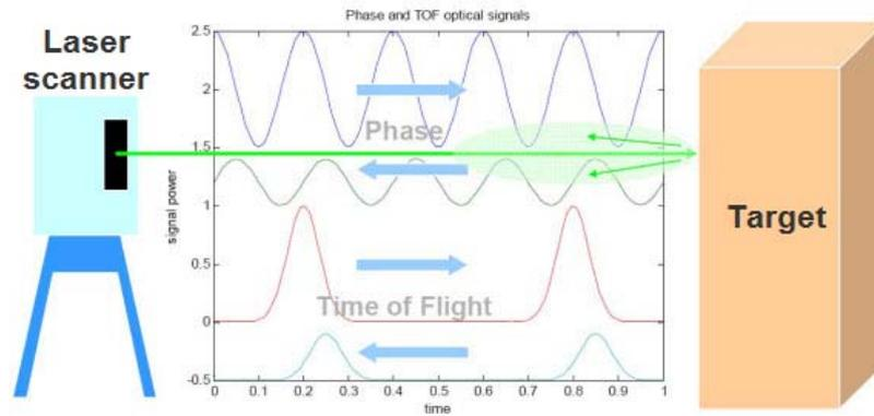
Figure 1. The operating principle of phase-based and time-of-flight 3D laser scanners. [2]
