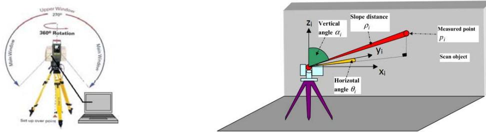
Figure 2. Spherical measuring system with a laser scanner system. [3]
