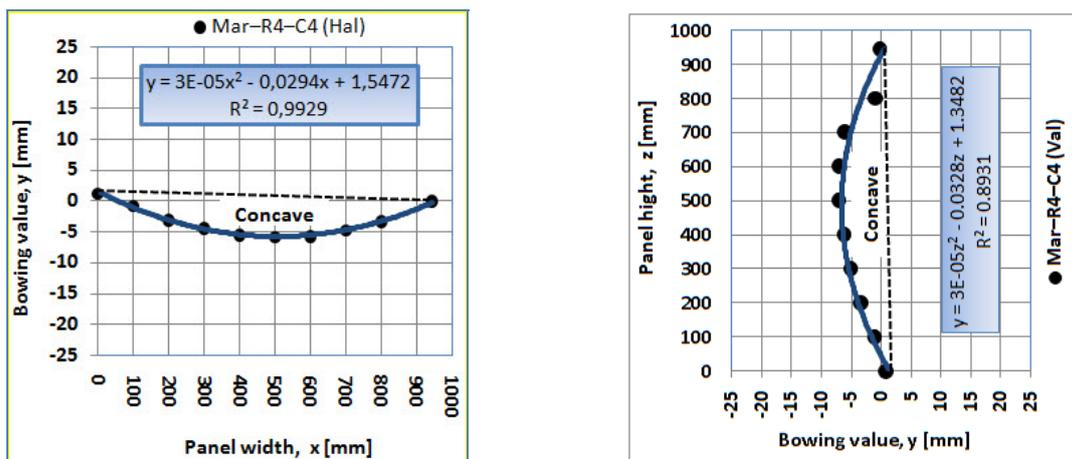
Figure 9. The manual measurements of the bowing of the marble panel Mar-R4-C4.
