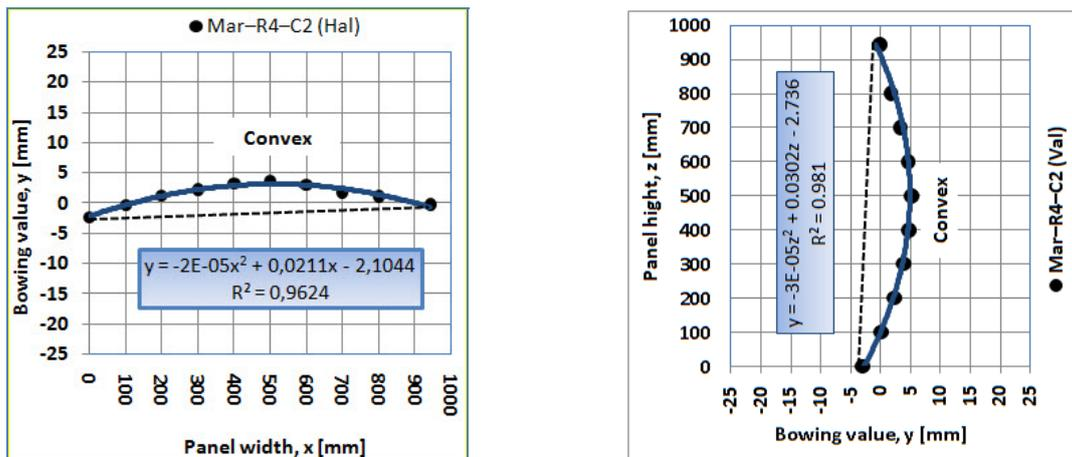
Figure 8. The manual measurements of the bowing of the marble panel Mar-R4-C2.
