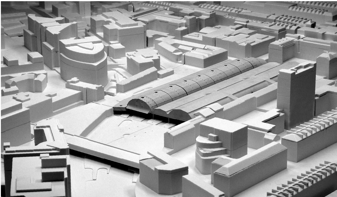
Fig. 5. Pressure tap tests of the Paddington Railway Station Span 4 Roof.
