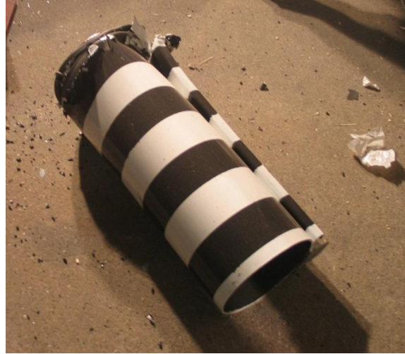
Figure 17. Steel missile after impact test.
