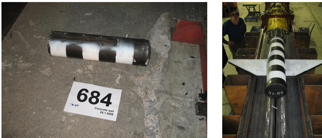
Figure 4. The rigid steel pipe missile with a diameter of 170 mm (left) and a 3D missile with wings (right).
