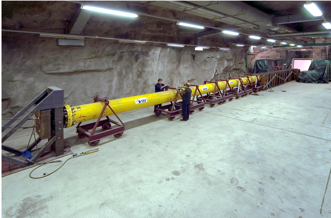
Figure 1. Impact test facility (pressure pipe, acceleration tube, piston catcher and force plate or impact wall)
