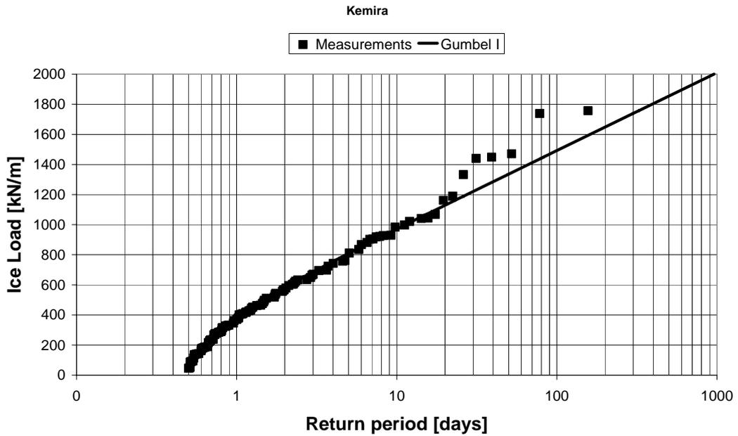
Figure 4. Measured long term ice loads onboard MT Kemira and Gumbel 1 distribution fitted on the data [8].
