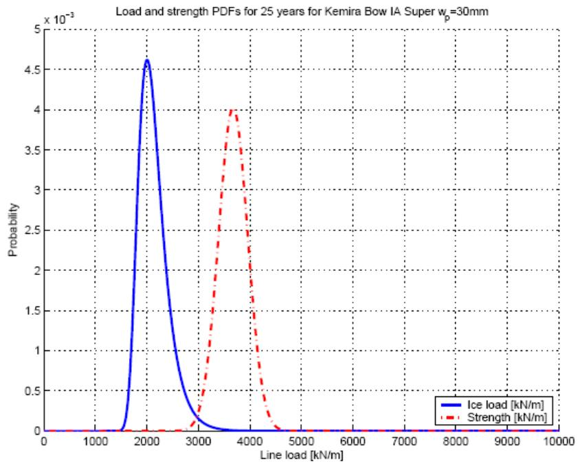
Figure 5. Obtained distributions for the strength and ice induced load.
