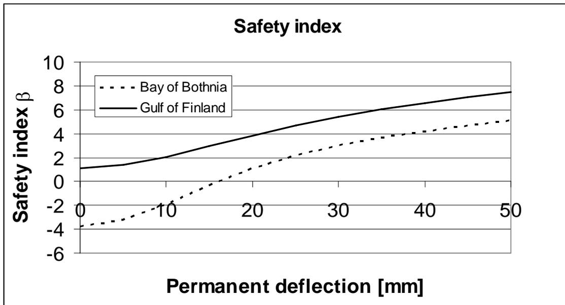
Figure 6. Obtained safety index as a function of the permanent deflection of the plating [12].
