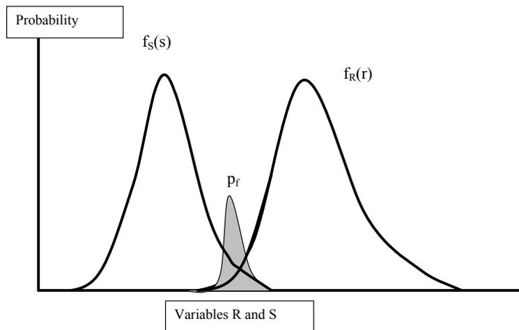
Figure 1. Illustration of the load, strength and failure probability distributions
