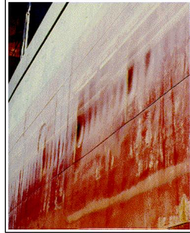
Figure 3. A typical ice damage [3]
