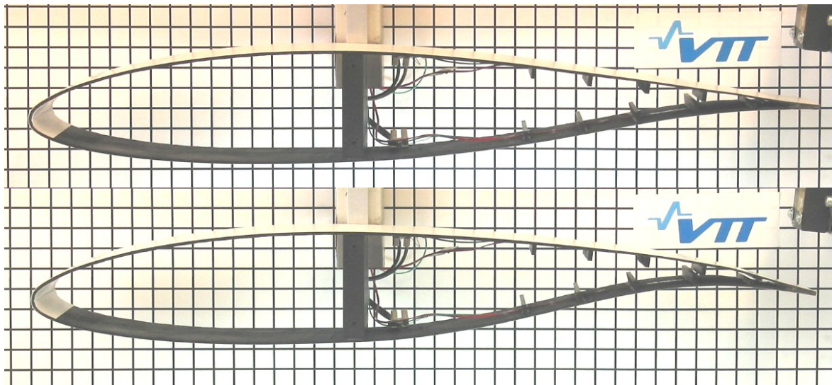
Figure 6. The airfoil and the test setup. Upper picture: non-active state, lower picture: activated state
