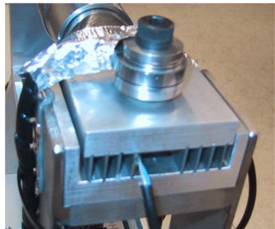
Figure 3. The SMA rib actuator. The bolt force sensor on the top.
