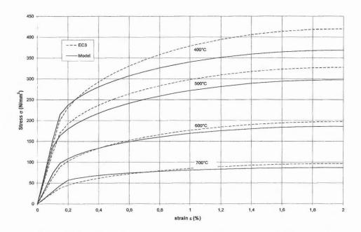
Fig. 6. Comparison between stress-strain curves of the modified model and EC3 for steel S420M at temperatures 400 °C - 700 °C.
