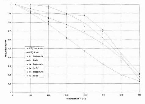
**Fig.4.** Reduction factors for elasticity modulus E(T), proportional limit  $f_p$  and yield strength  $f_y$  and  $f_x$  of steel S420M compared with the test results.
