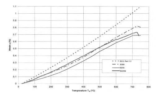
**Fig.2.** Thermal elongation determined for structural steels S235, S355 and S420M compared with thermal elongation according to EC3.
