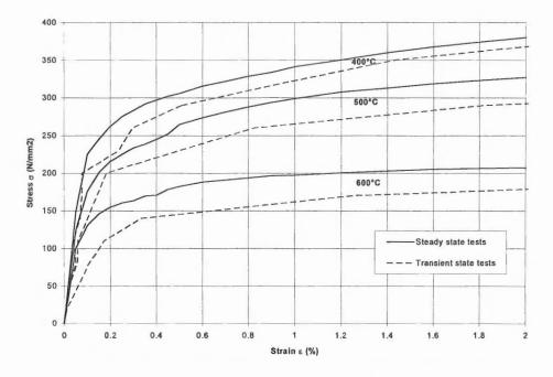
*Fig. 3 Measured steady state stress-strain curves for steel* S420M *at temperatures*  $400 \,^{\circ}\text{C}$ ,  $500 \,^{\circ}\text{C}$  *and*  $600 \,^{\circ}\text{C}$  *compared with the measured transient state curves.*
