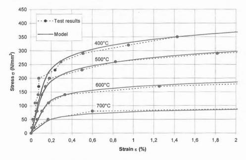
Fig 7. Stress-strain curves for steel S420M determined by using the modified Ramberg-Osgood model compared with the test results at temperatures 400°C - 700°C.
