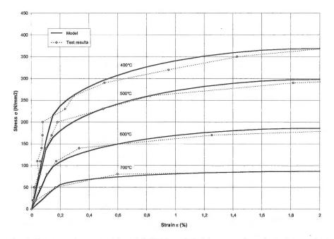
*Fig. 5.* Stress-strain curves of steel S420M modelled by using the calculation method given in EC 3 and compared with the test results at temperatures  $400^{\circ}$ C -  $700^{\circ}$ C.
