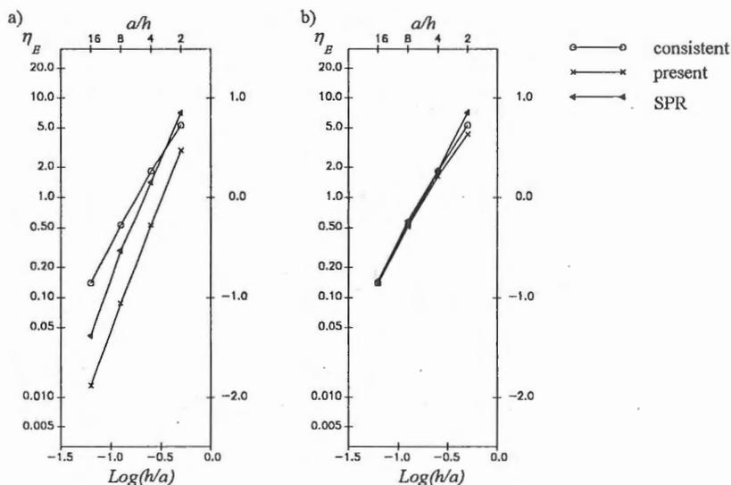
**Figure 2:** The circular hole problem with quadratic Lagrange quadrilaterals: (a) error of the smoothed and consistent solution (b) error estimate and exact error.
