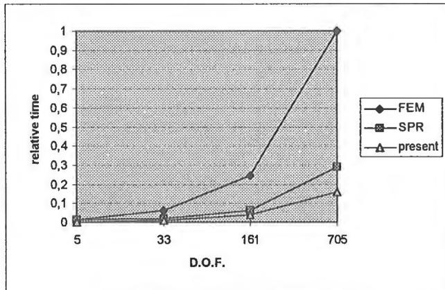
**Figure 7:** Relative computation time in quasi-harmonic square domain problem present and SPR-method compared to original finite element solution (*FEM*) using quadratic Serendip quadrilaterals.
