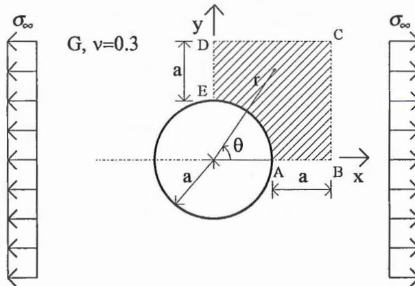
**Figure 1:** Infinite plate with a circular hole.
