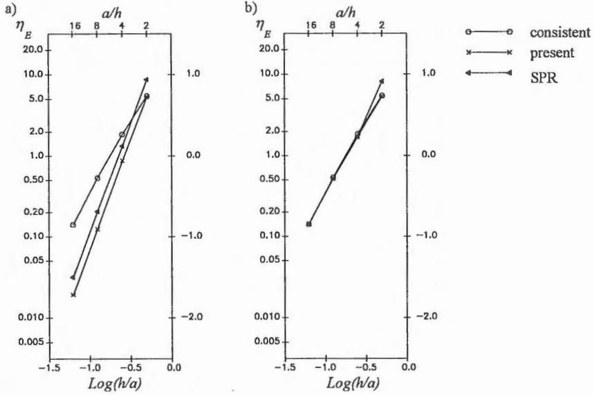
**Figure 3:** The circular hole problem with quadratic Serendip quadrilaterals: (a) error of the smoothed and consistent solution (b) error estimate and exact error.
