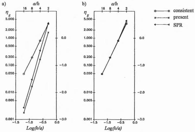
**Figure 6:** The square domain problem with quadratic Serendip quadrilaterals: (a) error of the smoothed and consistent solution (b) error estimate and exact error.
