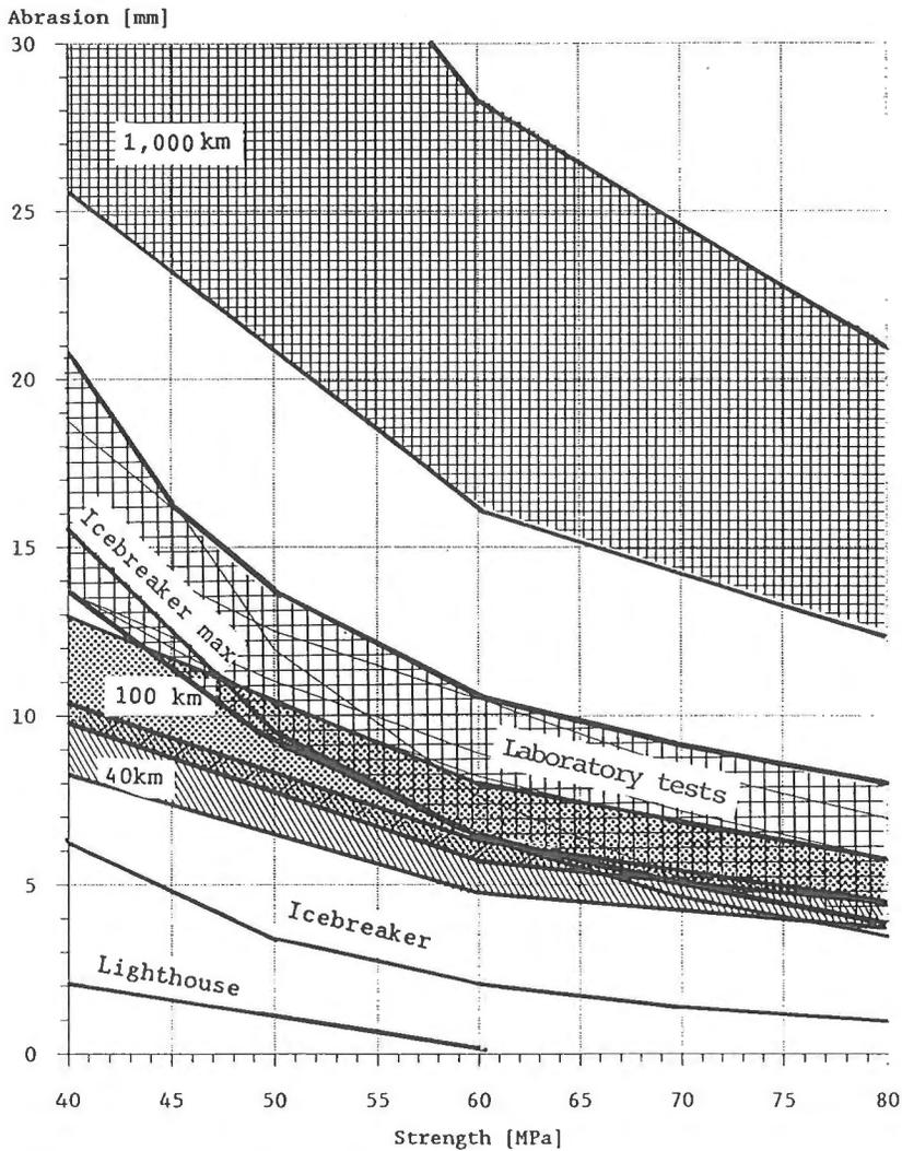
Fig. 9. Abrasion of concrete as the function of compressive strength /1/.
