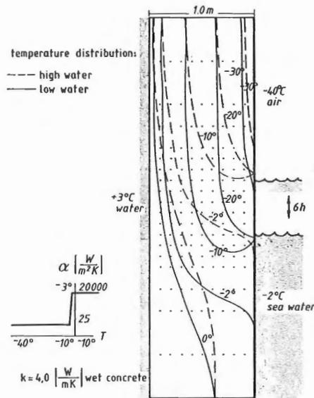
Fig. 12. Calculated temperature distribution during one tidewater cycle.
