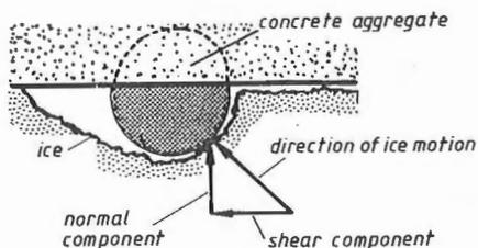
Fig. 5. Forces against protrudent aggregate stones /1/.
