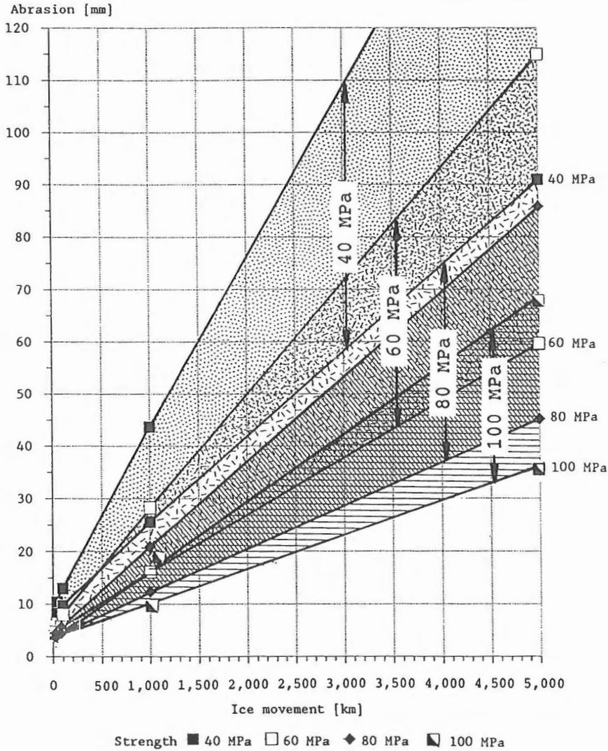
Fig. 8. Abrasion of concrete strengths  $f_c = 40, 60, 80$  and  $100$  MPa as the function of ice sheet movement /1/.
