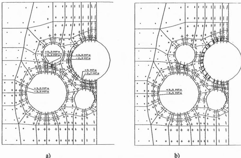
Fig. 10. Greatest stresses and cracks at a concrete temperature of  $-15\text{ }^{\circ}\text{C}$  ( $\Delta T = -25\text{ }^{\circ}\text{C}$ ) and tensile strength of the transition layer  $f_{ab} = 6\text{ MPa}$  (a-figure) and  $f_{ab} = 2\text{ MPa}$  (b-figure) /1/.
