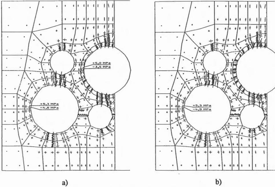
Fig. 11. Greatest stresses and cracks at a concrete temperature of  $-30\text{ }^{\circ}\text{C}$  ( $\Delta T = -40\text{ }^{\circ}\text{C}$ ) and tensile strength of the transition layer  $f_{ab} = 6\text{ MPa}$  (a-figure) and  $f_{ab} = 2\text{ MPa}$  (b-figure) /1/.
