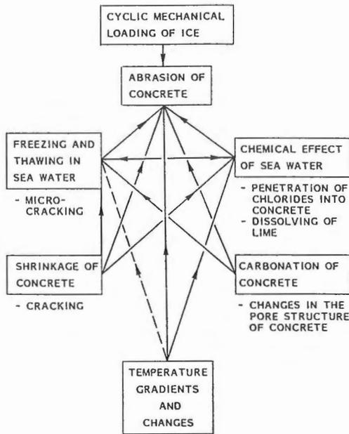
Fig. 1. Effects causing damage to concrete in sea water /1/.
