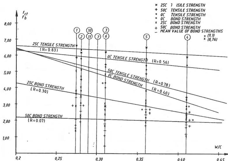
Fig. 4. Flexural tensile strength of concrete and the bond strength of aggregate stones as the function of the w/c ratio and number of freeze-thaw cycles /1/.
