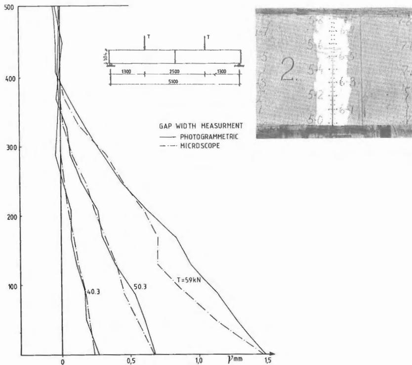
Fig. 8 Measured gaps  $\gamma$  of dry joint of prestressed concrete beam with unbonded tendons. Obs. linearity of  $\gamma$  in A.
