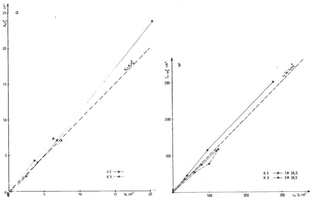
Fig 2. Test of prestressed granite beam with unbonded tendons, net area of section  $A_h$  and unbonded tendons
