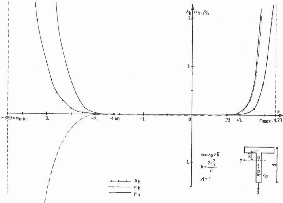
Fig 4. Deformation parameters of dry joint of T beam.
