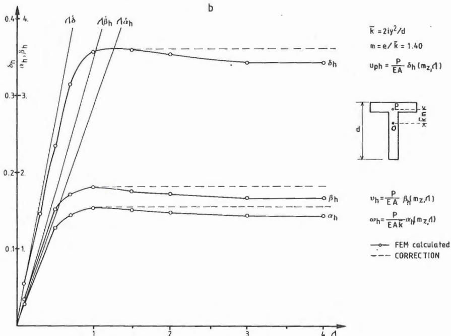
Fig. 5 Dilatation parameters  $\beta_h$ , rotation parameters  $\alpha_h$  and interpenetration parameters  $\delta_h$  versus slenderness ratio  $\lambda$ .
