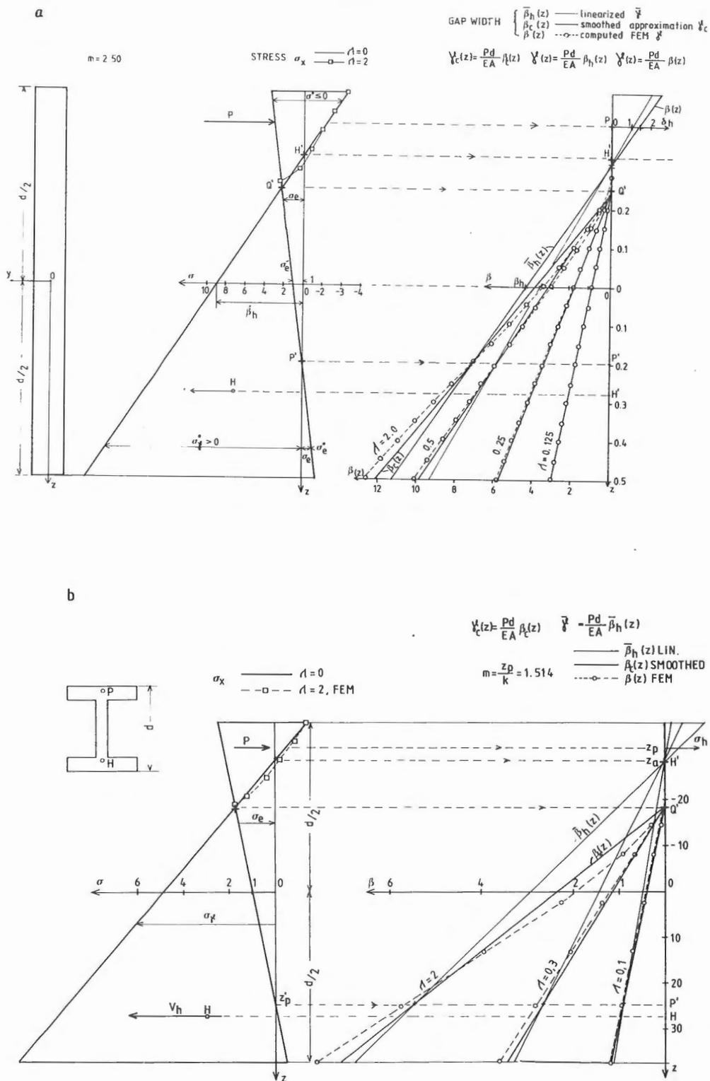
Fig. 7 Compressive stress distribution  $\sigma_x$  and geometric determination of relative gap width  $\beta_c(z)$  of dry joint.
