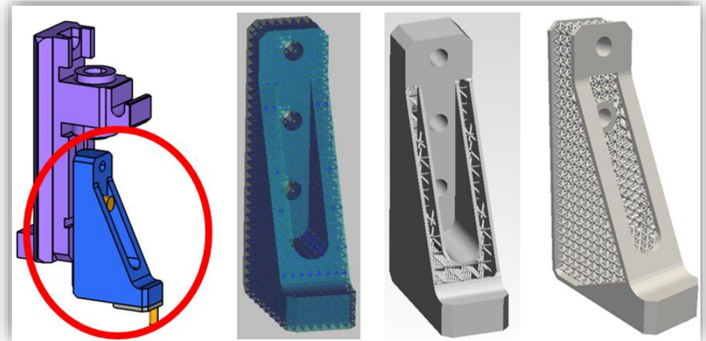
Example – lattice optimization of welding head bracket
