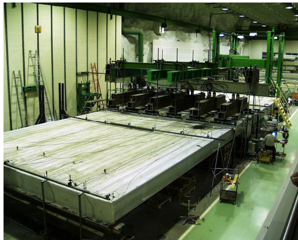
Fig. 122. Example of floor test. Size of test specimen 7,2 x 21 x 0,5 m 3 .
