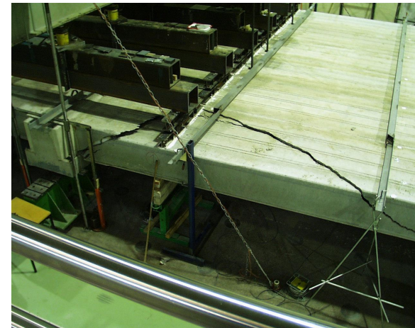
Fig. 123. Failure mode. The failure initiated next to the support of the beam.
